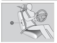
The side airbags are housed in the outside edge of the driver's, passenger's, and second row outer passenger's\* seat-backs.
