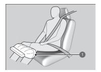
Deployed Passenger's Knee Airbag
