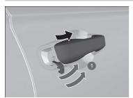
Unlock the driver's door with the key. Within 10 seconds of returning the key to the central position, turn the key in the unlock direction and hold it there.
