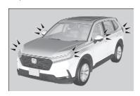
If the engine starts successfully, some exterior lights flash six times.
