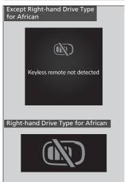
When the power mode is set to any mode other than OFF and you remove the keyless remote or card key\* from the vehicle and shut the door, an alarm will sound. If the alarm continues to sound, place the keyless remote or card key\* in another location.
