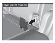
**3.** Remove the anchorage covers with the marks\* to expose the lower anchorages.
