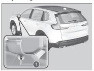
A camera in the passenger side door mirror monitors these areas and allows you to check for vehicles, in addition to your visual check and use of the passenger door mirror. You can also keep the system on for your convenience while driving.
