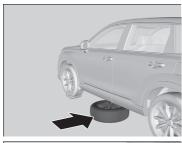
**8.** Place the spare tyre (wheel side up) under the vehicle body, near the tyre that needs to be replaced.
