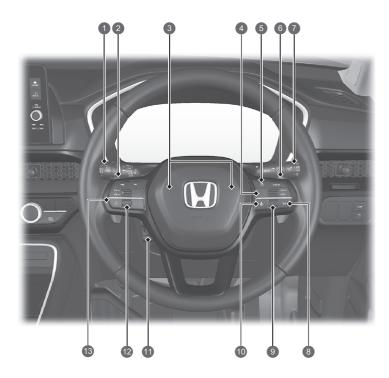
**1** ₩ Wipers/Washers\* ► P. 274 **■** Headlights/ → Turn Signals\* P. 262, 264 Fog Lights\* P. 266 LaneWatch\* >P.588 ② Paddle Shifter (Shift down)\* →P. 542 ⊕ Horn (Press the area around .) 4 LIM Button\* P.554 **⑤** Adaptive Cruise Control (ACC) with Low Speed Follow Buttons C>P. 626 6 Paddle Shifter (Shift up)\* →P.542 P. 262, 264 Wipers/Washers\* ←>P. 274 Fog Lights\* P. 266 LaneWatch\* P. 588 Button C>P.652 Interval Button ← P. 643 Steering Wheel Adjustments
