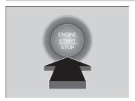
If you carry the keyless remote or card key\* and press **ENGINE START/STOP** button without depressing the brake pedal, the power mode will change in this order: VEHICLE OFF→ACCESSORY→ON→VEHICLE OFF
