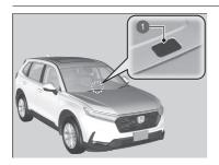
The automatic climate control system is equipped with a sensors. Do not cover or spill any liquid on them.
