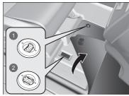
1 Unlock 2 Lock The driver's floor mat hooks over the floor anchors, which keep the mat from sliding forward. To remove a mat for cleaning, turn the anchor knobs to the unlock position. When reinstalling the mat after cleaning, turn the knobs to the lock position. Do not put additional floor mats on top of the anchored mat
