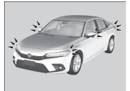
If the power system is turned off successfully, the exterior lights flash once.
