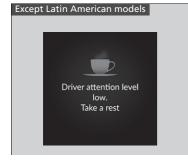
If one bar lights up, the **Driver attention level low. Time for a break.**\*1/**Driver attention level low. Take a rest**\*2 message will appear, a beep will sound, and the steering wheel will vibrate.
