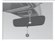
When you are driving after dark, the automatic dimming rearview mirror reduces the glare from headlights behind you. Press the AUTO button to turn this function on and off. When activated, the AUTO indicator comes on.
