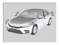
If the power system is turned on successfully, some exterior lights flash six times.
