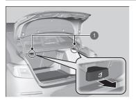
**1.** Pull the release lever in the boot to release the lock.
