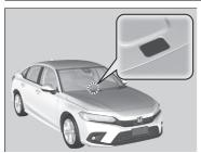
The automatic climate control system is equipped with a sensor. Do not cover or spill any liquid on them.
