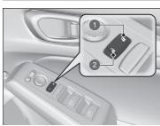
Press the master door lock switch in as shown to lock or unlock all the doors and the boot.
