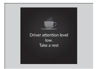
If one bar lights up, the **Driver attention level low. Take a rest** message will appear, a beep will sound, and the steering wheel will vibrate
