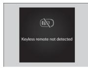
When the power mode is set to any mode other than OFF and you remove the keyless remote or card key\* from the vehicle and shut the door, an alarm will sound. If the alarm continues to sound, place the keyless remote or card key\* in another location.
