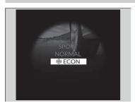
Facilitates fuel-efficient driving.
