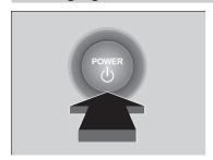
If you carry the keyless remote or card key\* and press **POWER** button without depressing the brake pedal, the power mode will change in this order: VEHICLE OFF→ACCESSORY→ON→VEHICLE OFF.
