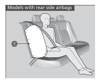
Deployed Side Airbag
